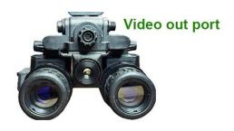
Connect the video out port to the Mini DVR AV in port with supplied video cable to record the images from the non-dominant eye tube
