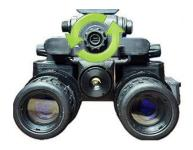
Turn the on/off switch clock wise to turn it on. Turn the on/oof switch counter-clock-wise to turn it off.
